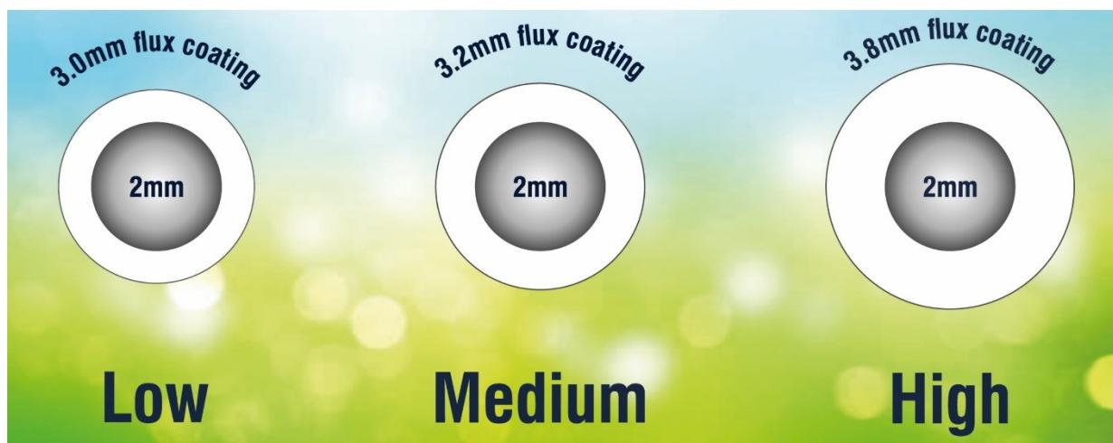
Flux coatings, on the example of a 2.0 mm rod
